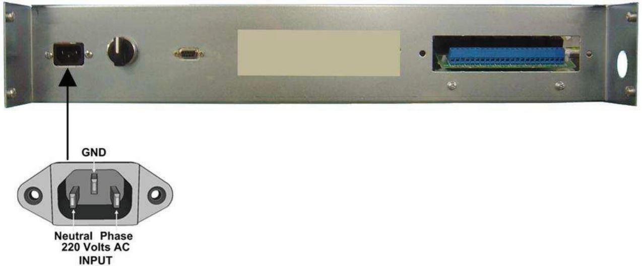
figure – 15 External power input
