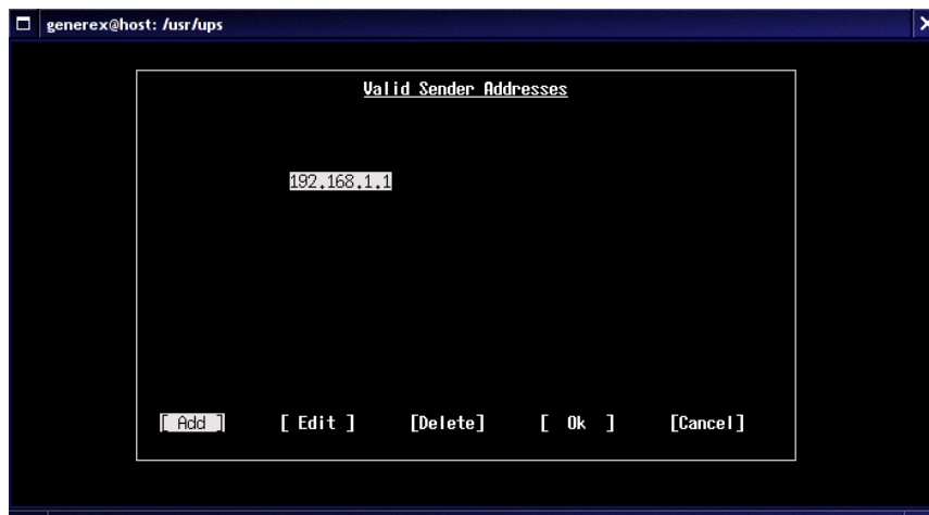
Figure 44 RCCMD UNIX sender overview
